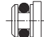
plug for 3/2 valve mounting CP-112 for G1/8, CP-9112 for G1/4 material: aluminium
